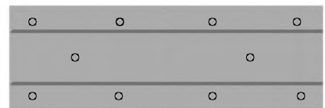
Top: Straight panel screw location.
