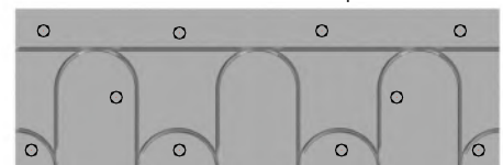
Below: Combo board screw pattern.
